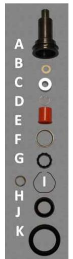
REBUILDING POT BEARING HOUSINGS: The used assembly is disassembled, cleaned and inspected. Epic **always** replaces the felt sealing washer (B), upper needle bearing (C), nylon spacer bushing (E), lower outer race (F), bearing cage (G), and wire retaining ring (I). Any static parts that show wear or faults are also replaced. The rebuilt assembly is lubricated with Kluber synthetic grease.
